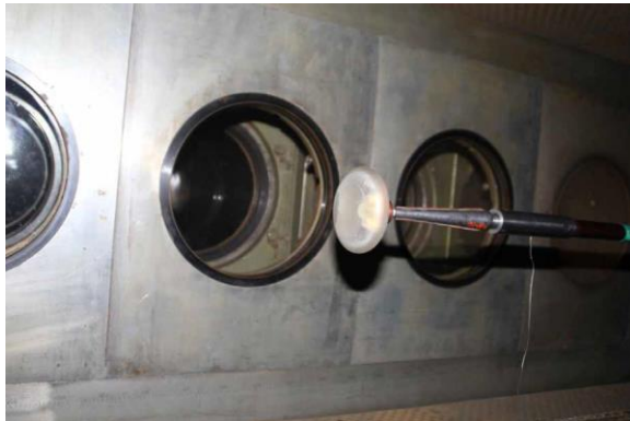
Figure 2: Lander mock-up model inside the wind tunnel during the RITD test program. Image: LA.
