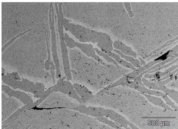
Figure 3: SEM-BSE image of an area of a polished sample; dark grey is kamacite; pale grey is taenite.
